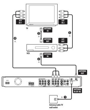
1 Connect your TV antenna/cable TV outlet to the ANTENNA IN (RF IN) jack on this recorder.
